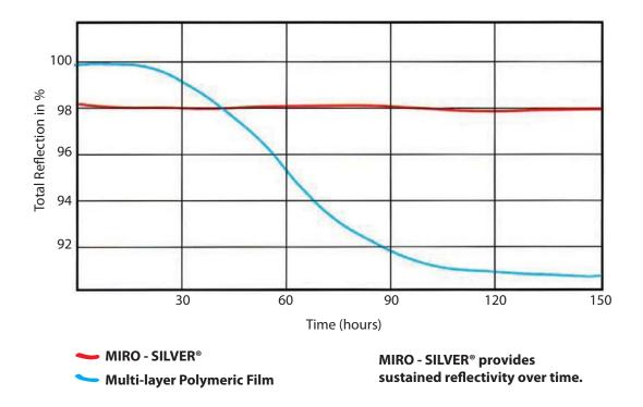
Sky Tunnel<sup>™</sup> utilizes Alanod Miro Silver<sup>®</sup> when producing the Rigid98 used in its Rigid Tube Kits. You can see from the graphic above, that whilst some other daylighting products using a Multi-layer Polymeric Film in their Rigid Tube have a higher initial Total Reflection, after just 40 hours of exposure to UV-C the reflection drops below that of the Miro Silver<sup>®</sup>.
